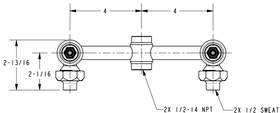
DIMENSIONS ARE IN INCHES AND AN APPROXIMATION OF A TYPICAL INSTALLATION
