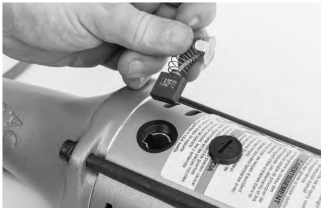
Figure 13 – Installation des balais
