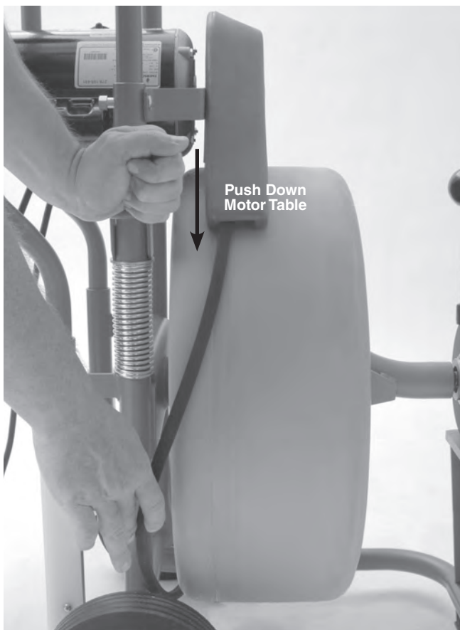
Figure 18 – Releasing Belt Tension
