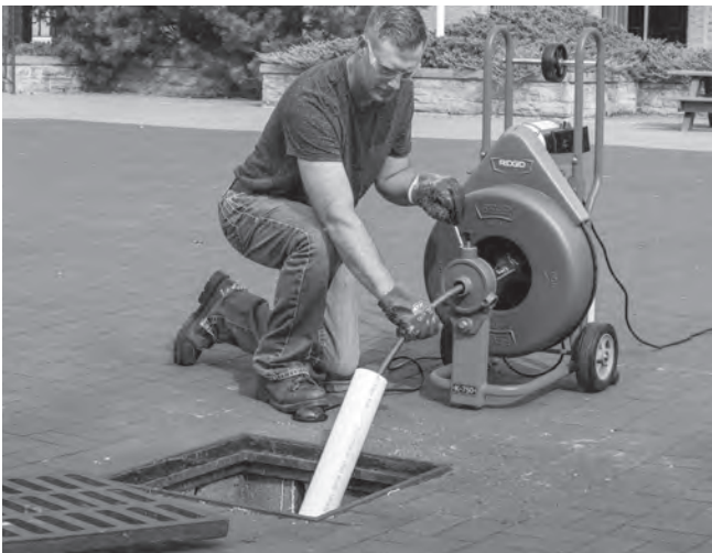
Figure 10 – Example of Extending Drain to Within 3' of Cable Outlet
