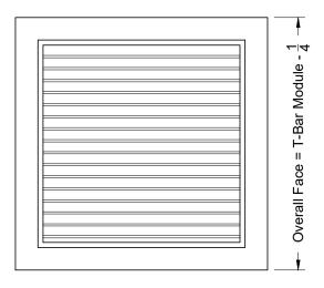
Note: This product complies with NFPA 90A-18 standard 4.3.7.3.2 and 4.3.8.3.2 and is constructed with openings through which a 1/2" sphere can not pass.
