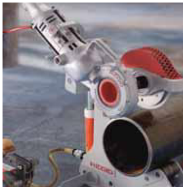
Model 258 Pipe Cutter with No. 700 Power Drive in use for cutting
