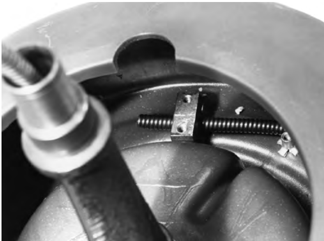
Figure 16 – Position New Cable Under Bracket
