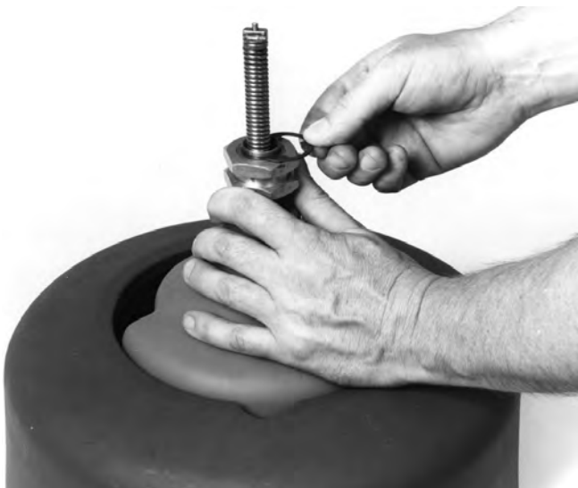
Figure 17 – Reassemble Inner Drum, Front Bracket and E-Clips
