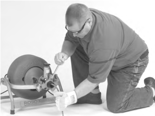
Figure 7 – Proper Operating Position
