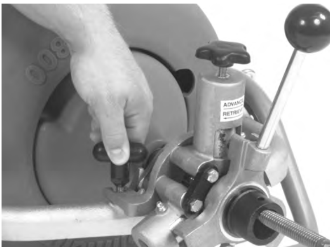
Figure 4 – Mounting the AUTOFEED Onto the Frame
