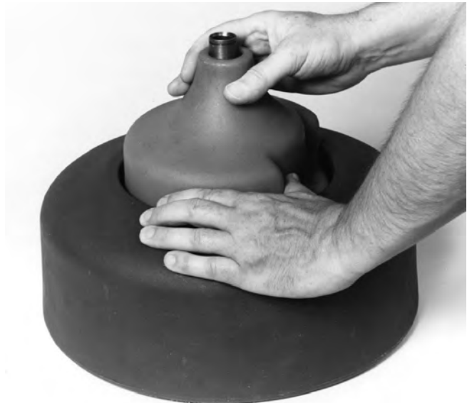
Figure 15 – Removing Inner Drum
