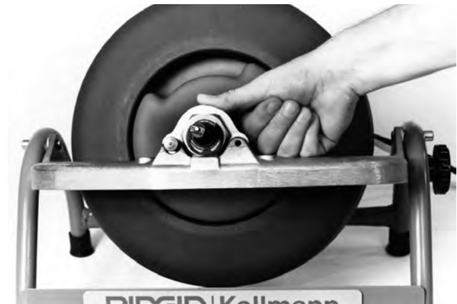
Figure 3 – Locking Front Bracket
