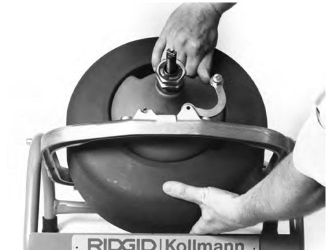
Figure 2 – Aligning Drum and Gearbox Bore
