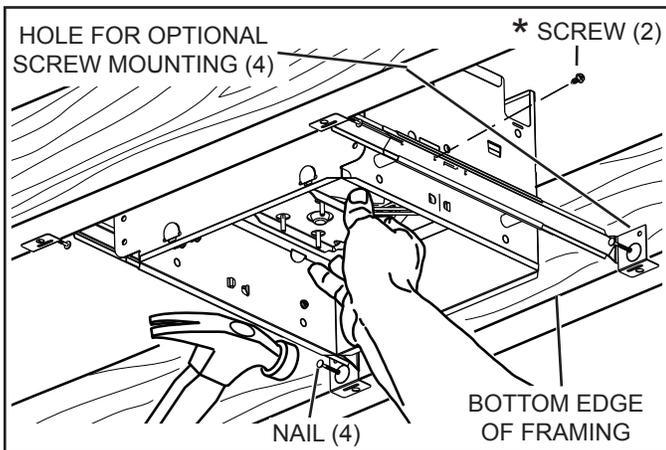
Extend HANGER BARS to the width of the framing. Hold ventilator in place with the hanger bar tabs wrapping around the BOTTOM EDGE OF THE FRAMING. NAIL ventilator to framing or fasten with screws (not provided) through HOLES near nails.
