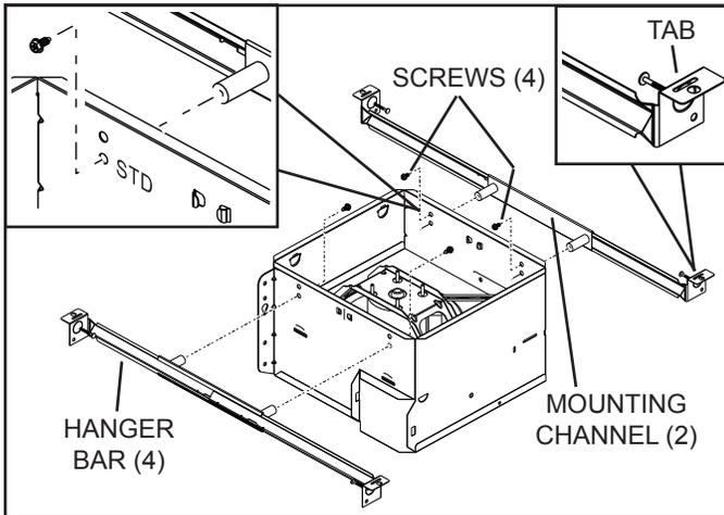
Attach the MOUNTING CHANNELS to the housing using the SCREWS supplied. Make sure TABS are oriented as shown. Use the set of mounting holes (marked "STD") to mount the housing flush with the bottom of the drywall. Use the other set of holes (not marked) to mount the housing flush with the top of the drywall.
