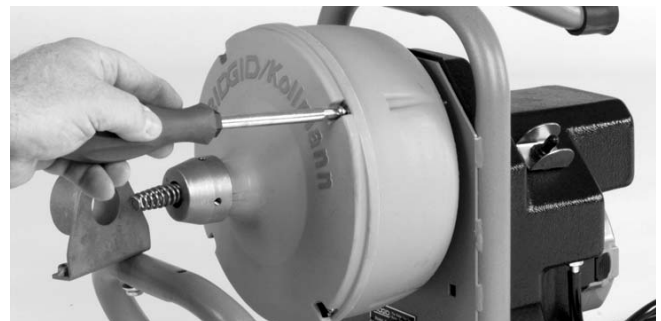
Figure 18 – Loosen 4 Drum Screws About 3 Full Turns But Do Not Remove
