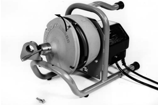
Figure 19 – Twist Drum Apart
