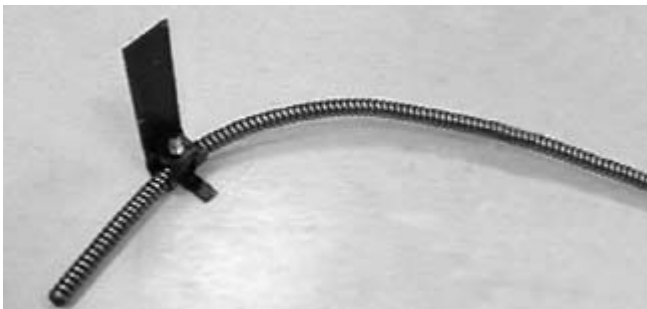
Figure 20 – Torque Arm Attached to Cable. Cable Should Be Permanently Bent as Shown with Clamp Installed Approx. 2" From End of Cable
