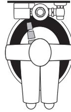
2. As the user enters the beam's effective range, 8" to 54" (203 mm – 1372 mm), the Object Lock Infrared Sensor senses the user.
