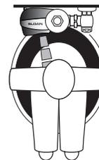
3. When the user steps away, the unit initiates a flush cycle. The unit then automatically resets and is ready for the next user.
