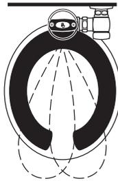
2. As the user enters the beam's effective range (22" to 42") the beam is reflected into the OPTIMA Plus Scanner Window and transformed into a low voltage electrical circuit. Once activated, the Output Circuit continues in a "hold" mode for as long as the user remains within the effective range of the Sensor.
