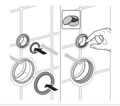
Remove protective sleeves from mounting rods.
