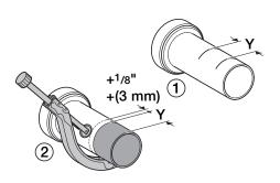
Bevel the sharp edges as shown to assure a smooth insertion into the pipe hubs in the wall.
