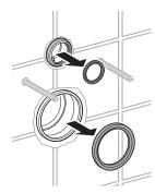
Insert discharge pipe into the pipe hub in the wall. Place a straight edge flush against the wall and mark a line on the pipe. Fit finned rubber seal onto flush pipe. Repeat same procedure for discharge pipe.
