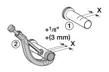
Add dimension Y and 1/8". Using that dimension, mark a line on the pipe measuring from the hub side. Cut off the pipe at the line with a pipe cutter.
