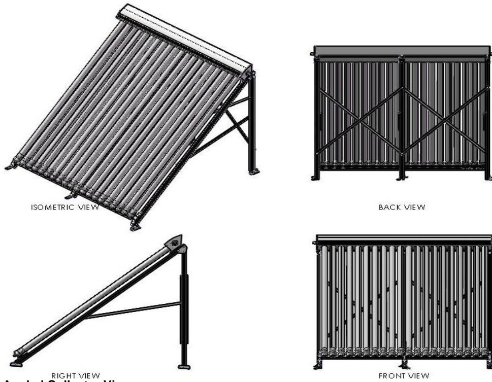
Figure 21 – Angled Collector Views
