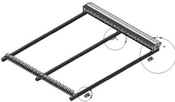
Figure 13 – Flush / Flat Mounting
