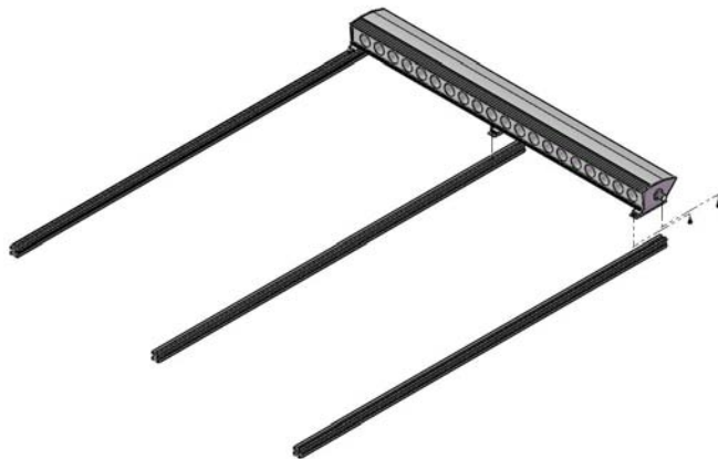
Figure 3 – Manifold and Base Tube Frame to Manifold Arms
