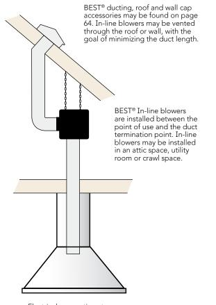
Electrical connections to both the hood and the in-line blower are required.
