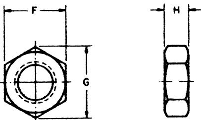
**Hex Jam Nut, double-chamfered**
