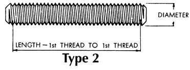
Continuous-thread studs are threaded from end to end and are often used for flange bolting with two nuts applied.
