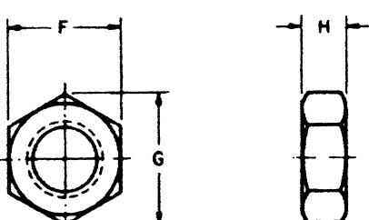
**Heavy Hex Jam Nut, washer-faced and double-chamfered**
