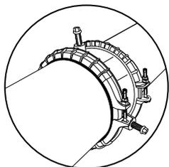
Positioning the Coupling for installation. If possible, place the coupling(s) on the replacement pipe (on both ends) and lower the pipe and couplings into the ditch. Slide the couplings outward so that they cover the minimum marks made in Step (4). Make sure there is sufficient space between the pipe ends inside the coupling so the centering pins do not touch the pipe and continuous dynamic deflection (CDD) can take place.
