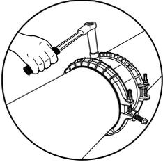
Set the centering pins. Secure the centering pins using an open-ended wrench or a socket wrench. Make sure the "o" ring on each centering pin seats properly beneath the pin head. Fully tighten the centering pins into the coupling body. The pins prevent the coupling from drifting along the pipe. They are not "set screws".
