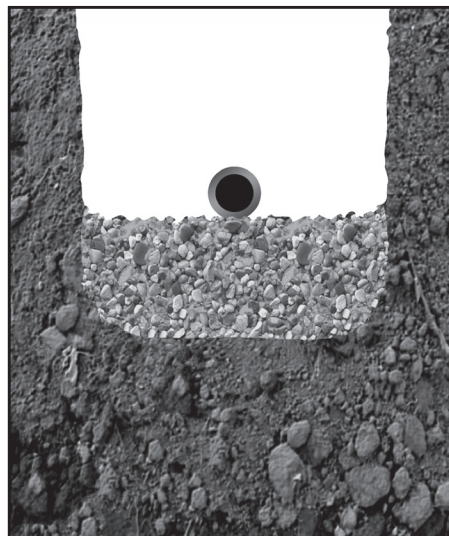
Trench in poor soil
