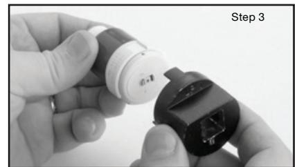
**Step 3.** Ensure that the TYCO W-Type 25 Installation Wrench is fully engaged onto the sprinkler. Fully insert all three Wrench Prongs into the slots on the sprinkler body.
