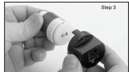
**Step 3.** Ensure that the TYCO W-Type 25 Installation Wrench is fully engaged onto the sprinkler. Fully insert all three Wrench Prongs into the slots on the sprinkler body.
