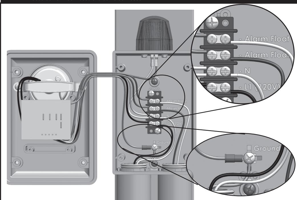
Refer to the Tank Alert® XT Terminal Block Option Installation Instructions for 8 position terminal block.
