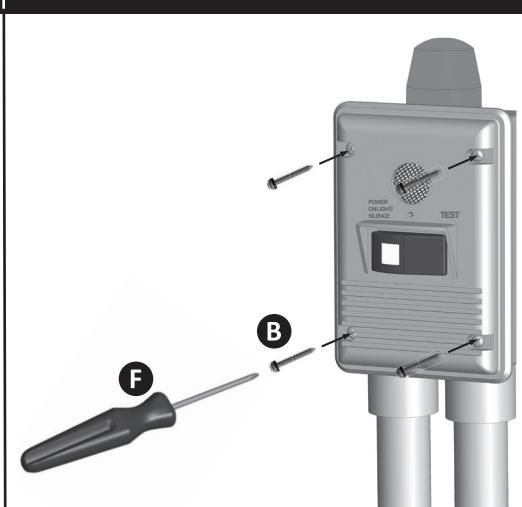
**6** Restore power and check alarm operation after installation (high level application shown).
