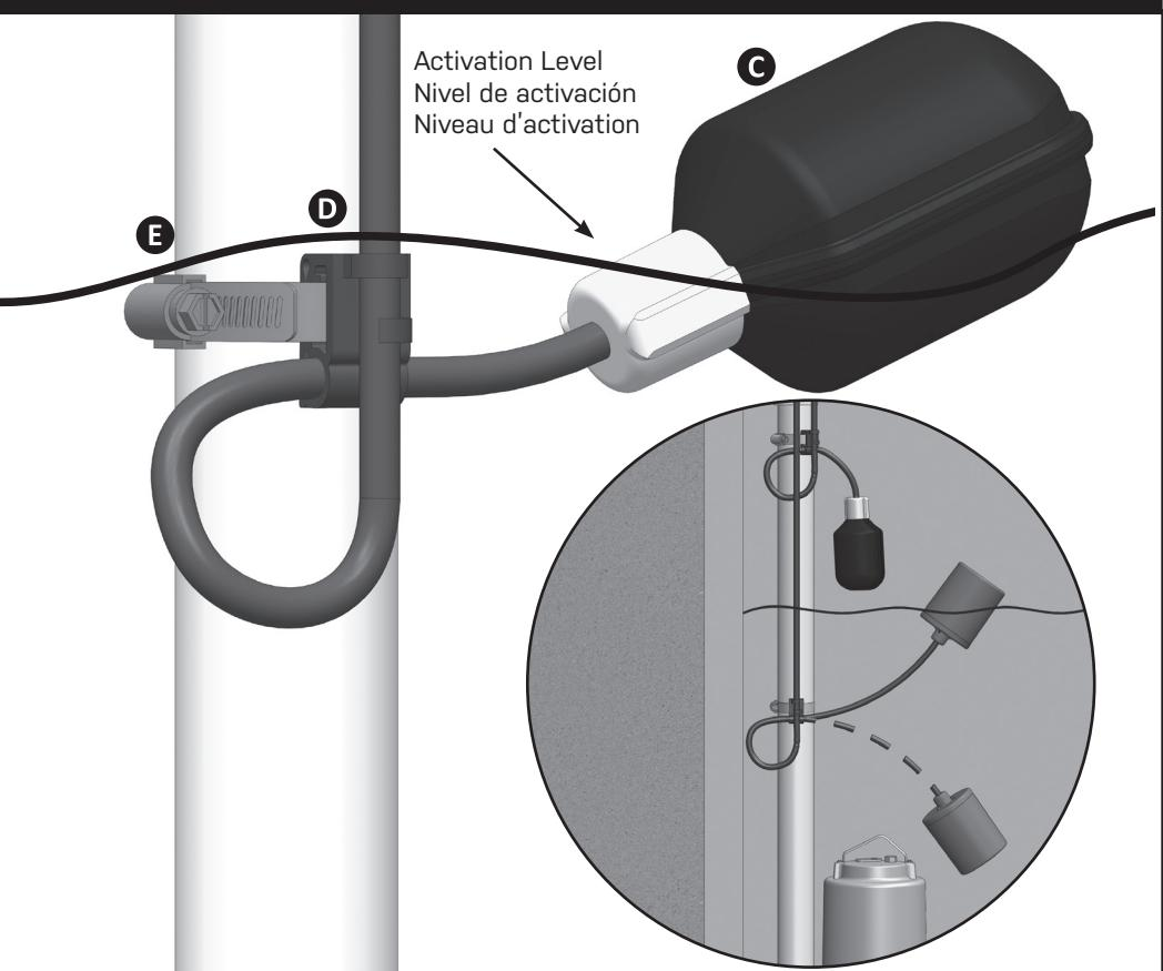
**3** Bring float switch and power cable through conduit and wire to 4 position terminal block. Connect ground wire to ground termination post.
