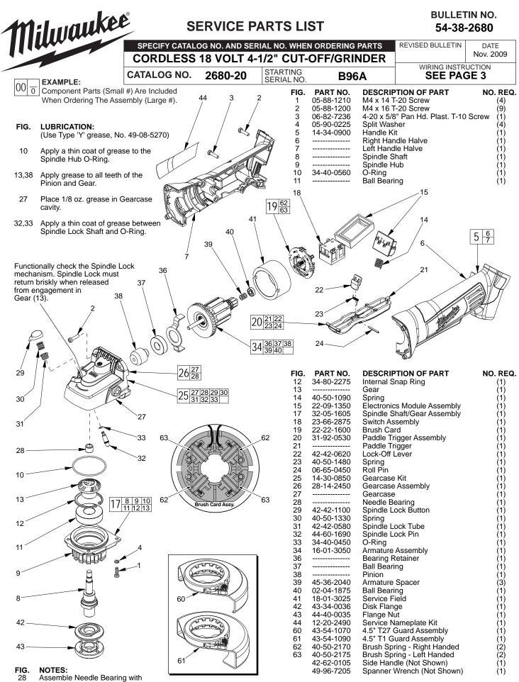
28 Assemble Needle Bearing with vendor I.D. facing the Gear.
