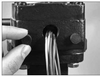
2. Remove the dust cap from the left side of the gear operator.
