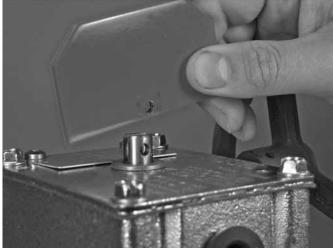
2. Remove the self-tapping torx screw (Item 5) from the actuator flag (Item 1). Remove the actuator flag (Item 1).
