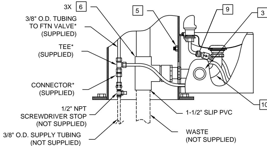
**\*NOTE: TEE SHOWN ASSEMBLED FOR REFERENCE ONLY. POSITION TEE AND TRIM TUBING AS NEEDED TO FIT INSTALLATION APPLICATION.**
