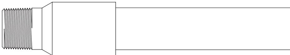
NOTE: THE TRANSITION FITTING AND THREAD CONNECTION SHALL BE PROTECTED FROM CORROSION BY FIELD APPLIED COATINGS OR WRAPPINGS. (EX. TAPECOAT® T-TAPE GPE)
