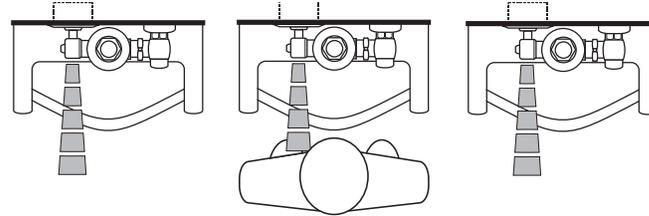
1. A continuous, invisible light beam is emitted from the OPTIMA® Sensor.
