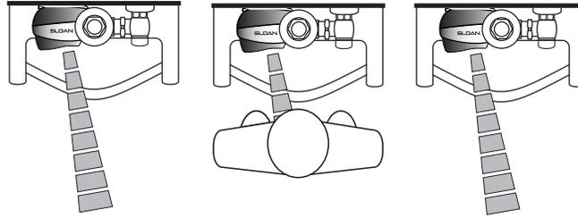
1. A continuous, invisible light beam is emitted from the SMOOTH® unit's Infrared Sensor.
