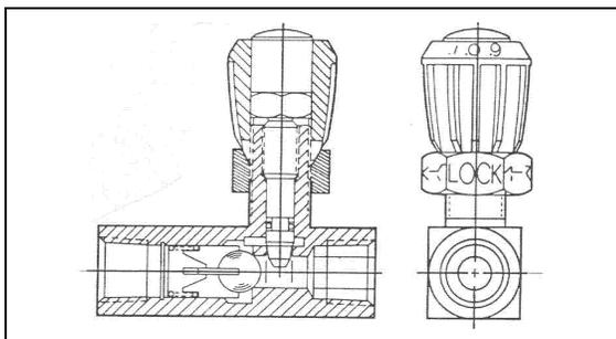
**Figure 2 – Flow Control Valve**
