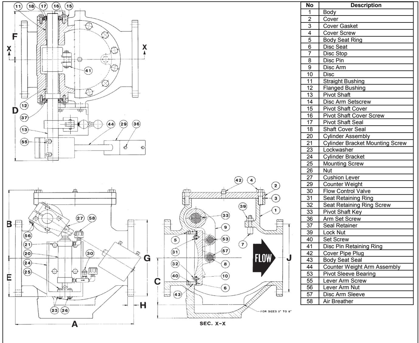
**Figure 7 – CVS-6000 Swing Check Valve (with Air Cushion Cylinder)**
