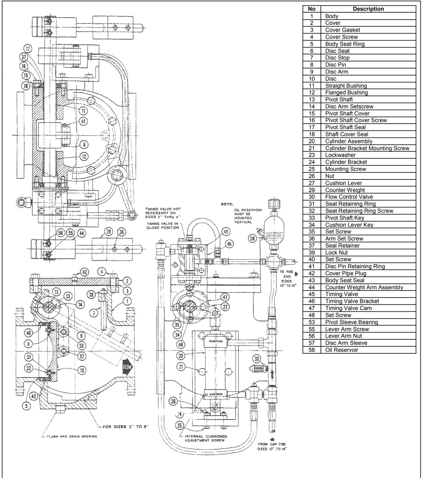
**Figure 9 – CVS-6100 Swing Check Valve (with Oil Cushion Cylinder)**
