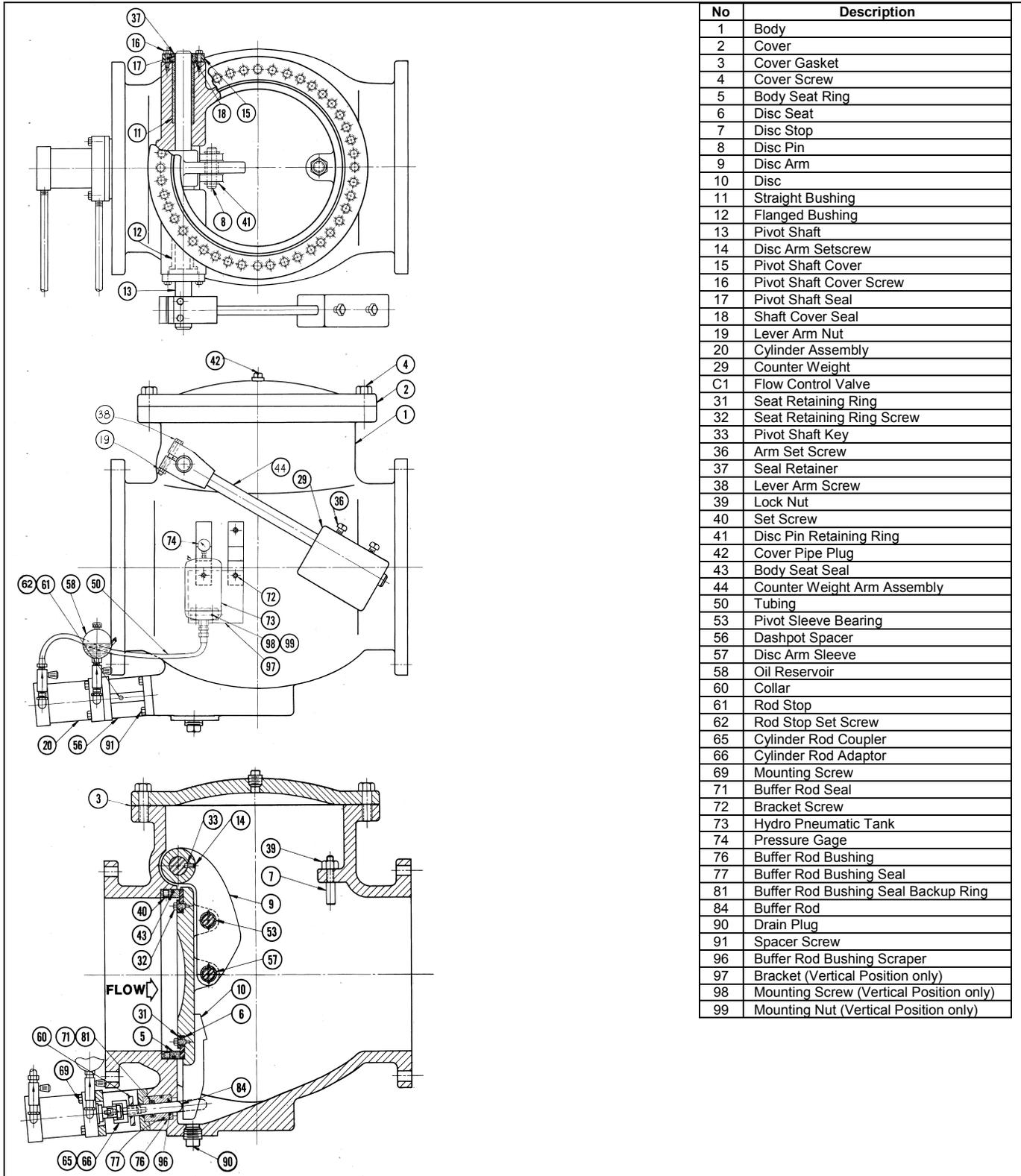
Figure 8 – CVS-6000B Swing Check Valve (with Oil Control Bottom Buffer)
