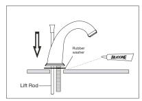
**B** Slip the spout mounting hardware back onto the spout. First the notched rubber washer, then the notched metal washer, wing nut, and brass lock nut.
