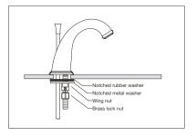
**C** Align spout and secure to the sink or counter surface by tightening the 2 screws on the wing nut.
