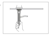
D Loop and connect the flexible hoses to the tee.
