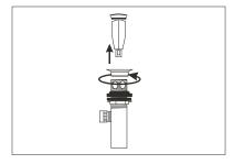
B Apply a ring of silicone caulking underneath the drain flange (do not use plumber's putty).
