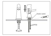
Slip the valve body's flexible hoses from the top of the sink or counter through the appropriate hole next to the spout. Aim the tee connecting hoses toward the tee connector.
