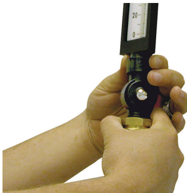
Rotate locking nut by hand.
