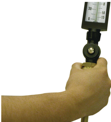
Grasp connection end firmly.
