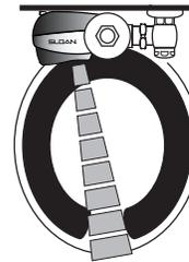
3. When the user steps away, the unit initiates a flush cycle. The unit then automatically resets and is ready for the next user.
