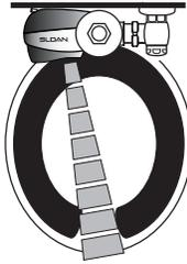
1. A continuous, invisible light beam is emitted from the OPTIMA® SMOOTH™ unit's Infrared Sensor.
