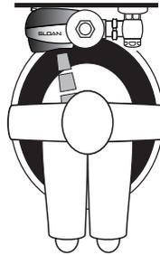
2. When the user enters the sensor's effective range, the Red LED light in the sensor window flashes for eight seconds. After eight seconds of sensing the user, the light will stop flashing and the unit waits for the user to step away before initiating a flush cycle.
