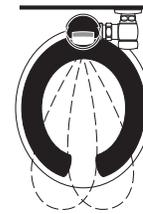
3. When the user steps away from the Sloan SOLIS® Sensor, the circuit waits 3 seconds (to prevent false flushing) then initiates an electrical signal that operates the Solenoid. This initiates the flushing cycle to flush the fixture. The Circuit then automatically resets and is ready for the next user.
