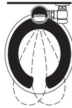
1. A continuous, invisible light beam is emitted from the Sloan SOLIS® Flush Sensor.
