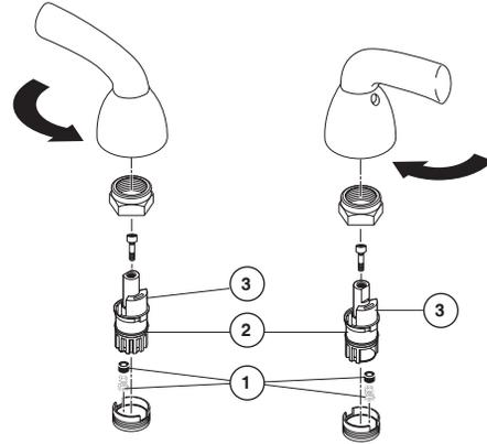
Remove Stream Straightener (1), turn faucet handles (2) all the way on. Turn on hot and cold water supplies and flush water lines for one minute.
