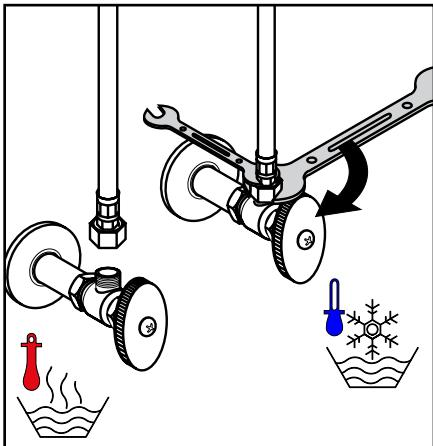
Connect the hot and cold supply hoses to the stops.
