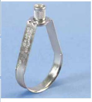
The 112 Swivel Loop Hanger, part of the CADDY® line of hangers, fasteners and supports from ERICO®, is ideal for suspending stationary non-insulated pipe lines, including CPVC pipes, in fire protection systems. The knurled insert nut helps simplify vertical adjustments, and the flared opening keeps the insert nut attached to the loop hanger at all times, providing added convenience and eliminating the frustration of dropped nuts.
