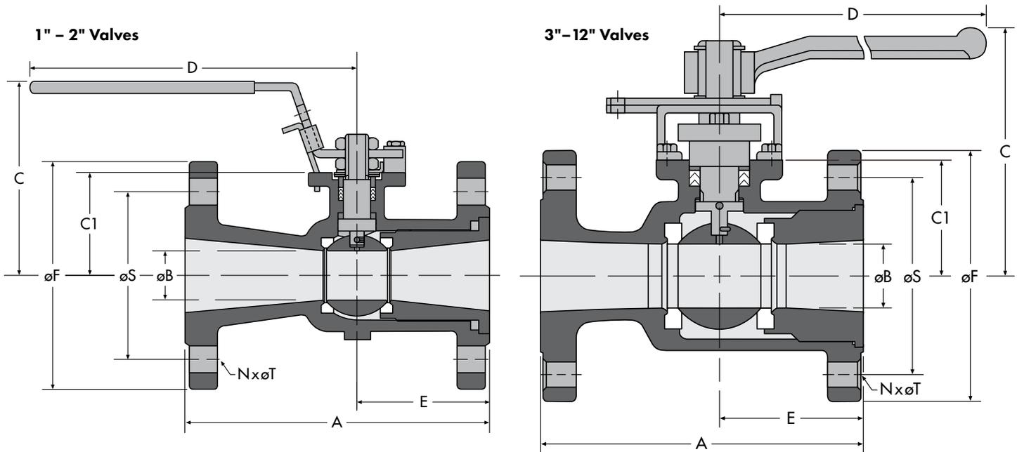
**NOTE:** Gear Operators are suggested on size 10" and 12" valves.
