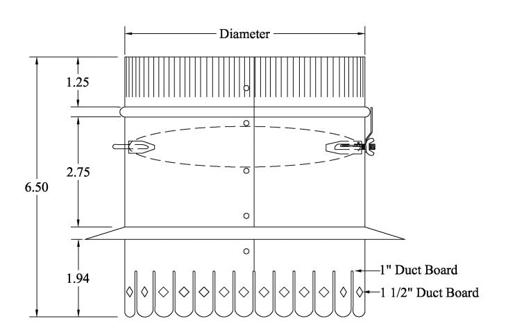
PART #: 507D(Size) DESCRIPTION: Round metal starting collar w/damper for Ductboard
