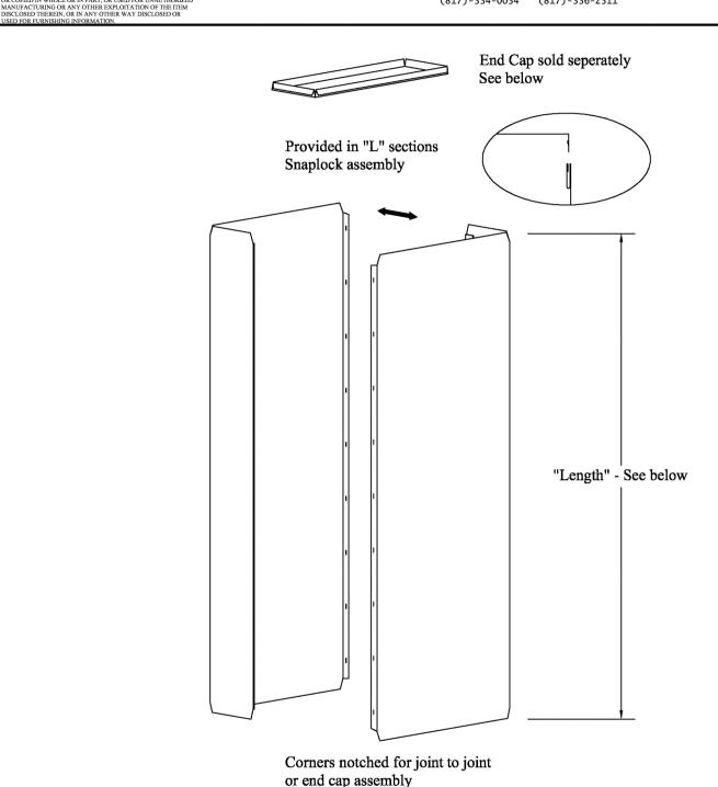
PART #: V-WS10(length) DESCRIPTION: Wall stack duct
