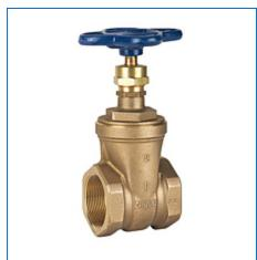
**Specifications UPC** Code 039923617521 Type Gate Valve **Valve Size** 3 T -- Female NPT Thread (FIPT) **Connection Type Seat Material Bronze** Material Bronze T133 3 THD 150# NRS GATE BRZ **Description Valve Operator** Standard Handwheel **Turns/Operation** Multi-Turn Weight 14.864 lb
