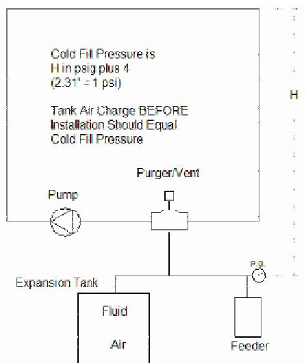
As an example, the CSFP for a system with a static height above the fill point of 40 feet would be:  $(40/2.31) + 4 = 21.3 \text{ psig.}$
