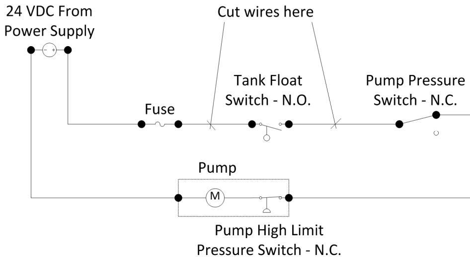
2. Connect the wires to complete the circuit without the float switch.
