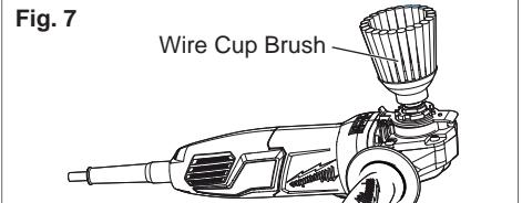
**WARNING** Because the wires on wire wheel brushes are directed towards the operator, a guard must be used to protect the operator when fatigued wires break.
