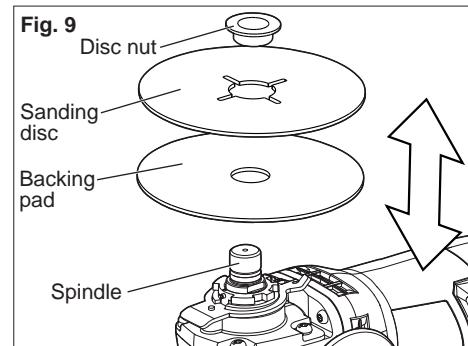
4. Place sanding disc on backing pad and secure assembly to spindle with disc nut.
