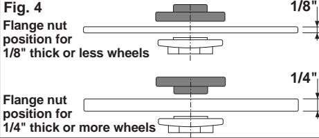
6. Position the flange nut over the spindle according to wheel thickness (Fig. 4).
