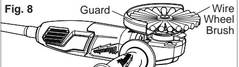
Test wheel for balance and loose or damaged wires by letting it spin for one minute before applying it to the workpiece. During this time, no one should stand in front of or in line with it.
