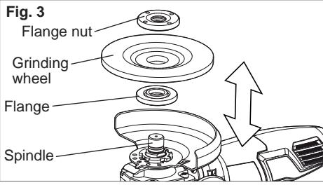
5. Place the selected wheel on the spindle and align it with the flange.
