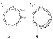
A. Halogen light control B. Fan control
