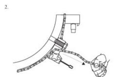
Pull the chain through the chain tensioner above (top) the cam making sure that the round end of the cam is facing out while the toothed "sharp" end is facing toward the valve.
