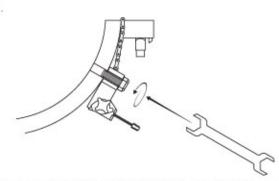
Use a restraint bolt to attach the chain drive unit to first restraint bolt hole on the lower half of the valve, on the opposite side of the cutting port.
