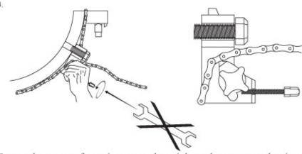
Rotate the cam as far as it can go, then tighten the screw so that it presses against the round end which will tighten the chain and prevent any slipping. It is important that you DO NO USE A WRENCH to tighten the screw, using a wrench can cause extra strain on the drive chain and on the gearbox.
