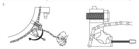
While keeping tension on the chain, rotate the cam so that the toothed end catches between two links. You may have to loosen it one or two links for the tooth to catch.
