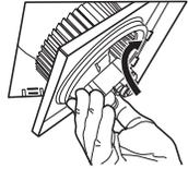
8. Pivot blower up into housing until single tab of blower snaps into single slot of housing.
