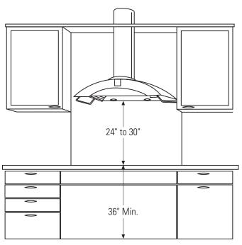
The vent hood must be installed 24" min. and 30" max. above the cooking surface depending on the ceiling height.
