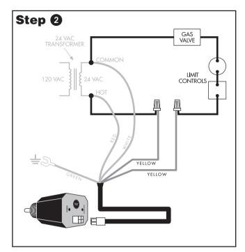
Cut-off the connectors and strip the ends of the two yellow wires of the Model 1100 harness. Break into the burner circuit between the *hot* side of the transformer (R) and other limit controls. Connect either YELLOW wire to the *hot* side. Connect the other YELLOW wire in series with other limit controls. Important: The switch contacts of the low water cutoff (yellow wires) must be wired in series with all other limit and operating controls (as shown above).
