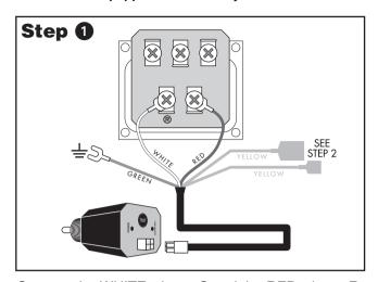
Connect the WHITE wire to **C** and the RED wire to **R** using the screw terminals on the control center.
