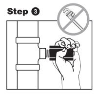
Hand tighten the control into boiler tapping or pipe tee. Be careful not to cross thread.
