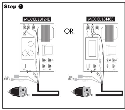
Connect the WHITE wire to **TV** and the RED wire to **Z.** Connect the GREEN wire to the ground screw on the bottom of the aquastat or any other suitable, unpainted ground screw. **Note:** for operation of the control, the green wire must be connected to a ground source electrically common with boiler ground.
