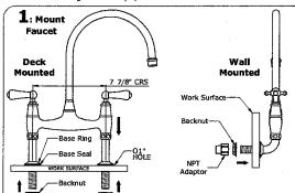
Ensure the mixer is orientated correctly, levers should rotate to point forward. After removing backnuts, place complete faucet through  $\emptyset1$ " holes at 7. 7/8" centers (do not remove unions from body) - product is fitted with straight unions, distance must be exact. Secure mixer with a suitable faucet wrench.
