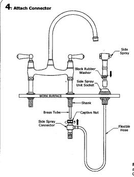
The side spray connector must be installed on the hose before mounting on the cold side shank.
