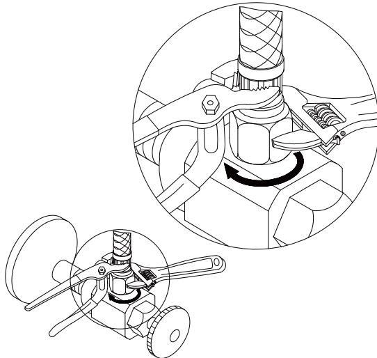
**5. IMPORTANT!** Tighten the hose onto water supply. Use two wrenches to avoid twisting hose when tightening.
