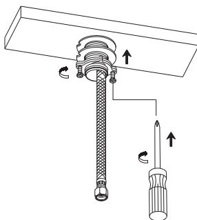
3. Insert faucet into 1 1/2" diameter mounting hole in deck. From underneath the sink, install the washers and lock nut.
