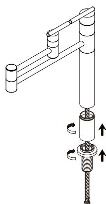
1. Install the mounting shank assembly onto the body tube. Note: If faucet height is satisfactory for your installation, go directly to step 3 below. If faucet height must be raised, install 3" extension tube (supplied) per step 2.
