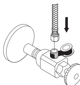
4. The supply hoses fit 3/8" supply valves. Apply pipe sealant tape to threads on valve before attaching the supply hose.
