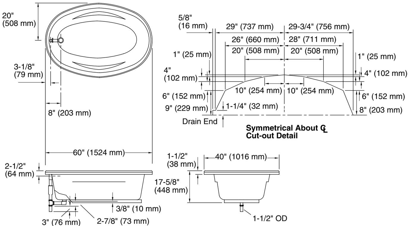
No change in measurements if connected with drain illustrated. (K-11677 or K-11677M)
