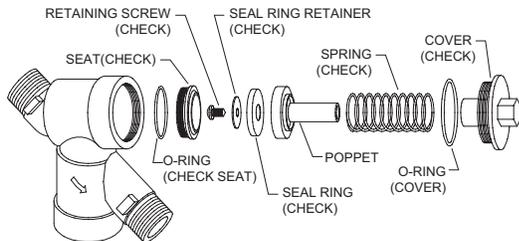
To remove seal ring, remove screw and seal ring retainer. If the reverse side of the seal ring is unused, it is possible to invert the seal ring. This would be considered a temporary solution to fixing a fouled check and should be replaced with a new seal ring as soon as possible.
