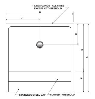
It is recommended that a floor drain at or near the entrance be included. These floors must be set on groutbed in order that floors be level.
