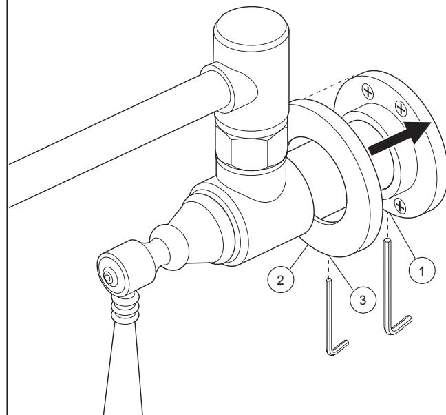
**E.** Wrap plumber tape (1) around pipe threads. Install the gasket (2) and the flange (3) using the 4 screws (and anchors if required) provided.
